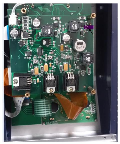
3. On the right side of the power board you will find the R6. Please replace the R6 with the parts with value of 3.4kohm, 0805 package. If can't find an 0805 package, you can use a 0603 package which is slightly smaller, just have add a little more solder, but do not add to much solder to avoid shorting the next component, R5,U3 or C18.
