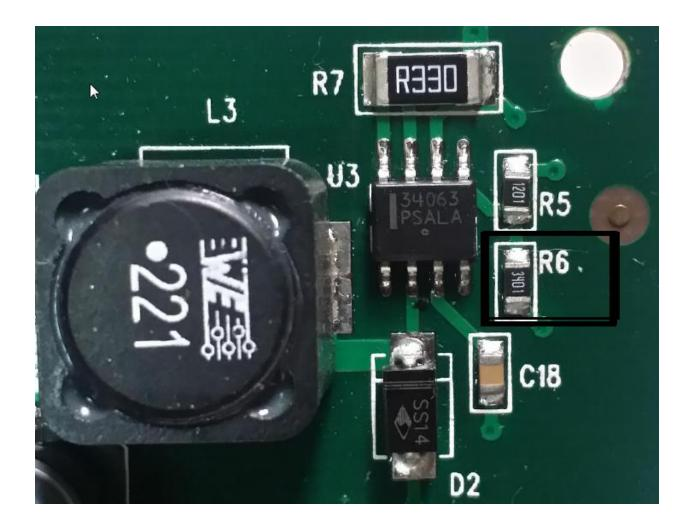
4. After replacing the R6, you should be able to use the new socket adapter.
